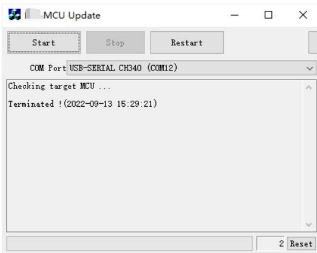
5) Connect the equipment to the computer via USB cable(Do not connect the power cord).After displaying the same information as the picture, click "Start".Finally, plug in the power cord.
